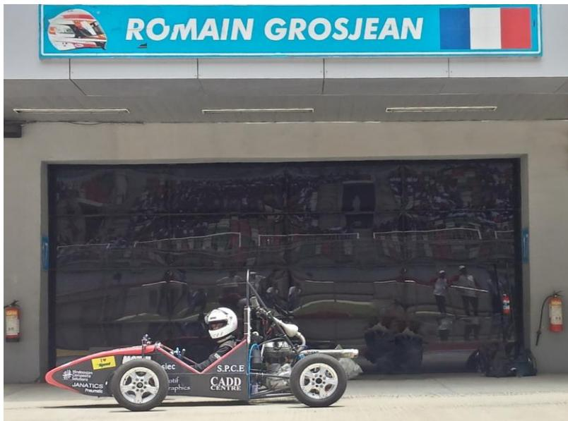
achieved major weight reduction due to self-manufactured carbon fiber nose and panels and optimization of wheel assemblies and drive train components which ultimately resulted in a better fuel economy.
